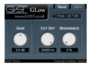
The three knobs are presented the same way for consistent and easy identification. Above each knob, its function is labelled. Below each knob, a numerical readout reflects the user adjustments or allows the user to manually specify exact values. In addition to the controls, there is a display showing the peak level of the outgoing signal, in decibels.
