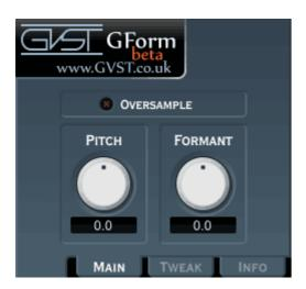
The main user interface is straightforward with just three variables - pitch, formant and an oversample switch.
