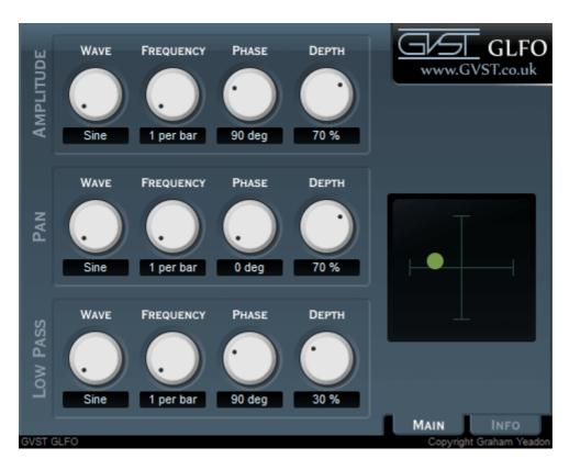
The controls are in three groups of four, each group controls one of the three LFOs.
