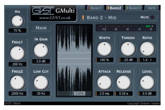
Each knob is laid out the same way for consistent and easy reference. Above each one, its function is labelled. Below each is a numerical readout of its value. There is also a waveform display and a gain reduction meter for each band.
