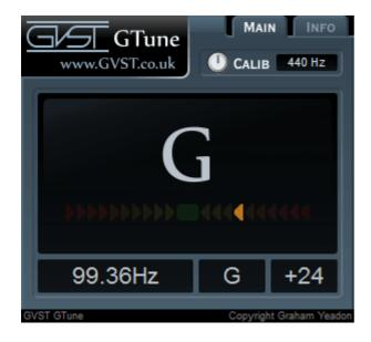
The user interface has four parts. From top to bottom these are the reference frequency control, the main display, the coarse-tune "LED" indicators and the frequency readout.
